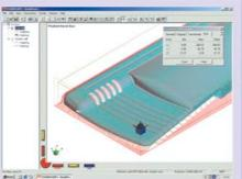
user to choose between standard 3 axis milling - x,y,z or 'Barbecue milling' - x, z, a, the third axis rotating the model, as on a spit, for milling!
