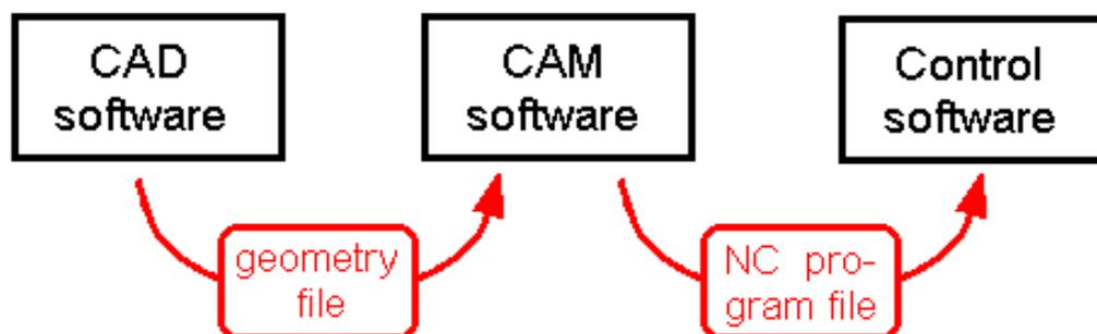
In order to manufacture a part, nowadays typically three different software programs are used (see the illustration above):
