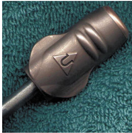
Figure 6: This electrode, to create the cavity in a production mould, was milled using DeskProto. It has been used for the mouthpiece presented in Case 3 (courtesy of Molds Direct and Ultimate Direction).
